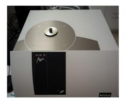
Thermodynamic parameters associated with a variety of materials such as specific heat, entropy and enthalpy change can be assessed. This helps in distinguishing crystalline and non-crystalline materials. The phase transitions associated with plethora of materials can be ascertained.
